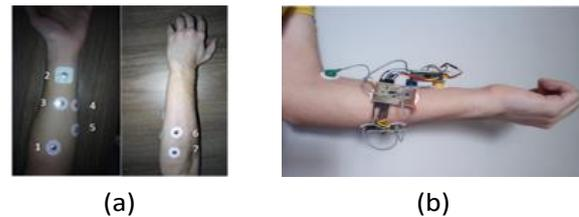
**Figure 2.** (a) Position of the electrodes on the forearm, (b) the device on the forearm
