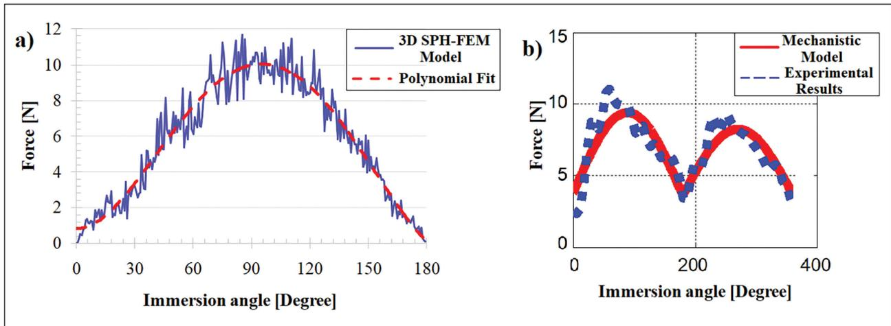
**Figure 3.** (a) Planar resultant force simulated with proposed 3D SPH-FEM model, (b) Experimentally measured and analytically calculated planar resultant force [depth of cut  $100\mu\text{m}$  and feedrate  $10\mu\text{m}/\text{rev-tooth}$ ].
