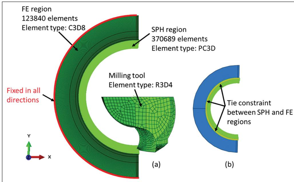
**Figure 1.** (a) 3D SPH-FE model of micro-milling of Ti alloy (b) Details of tie constraint imposed.
