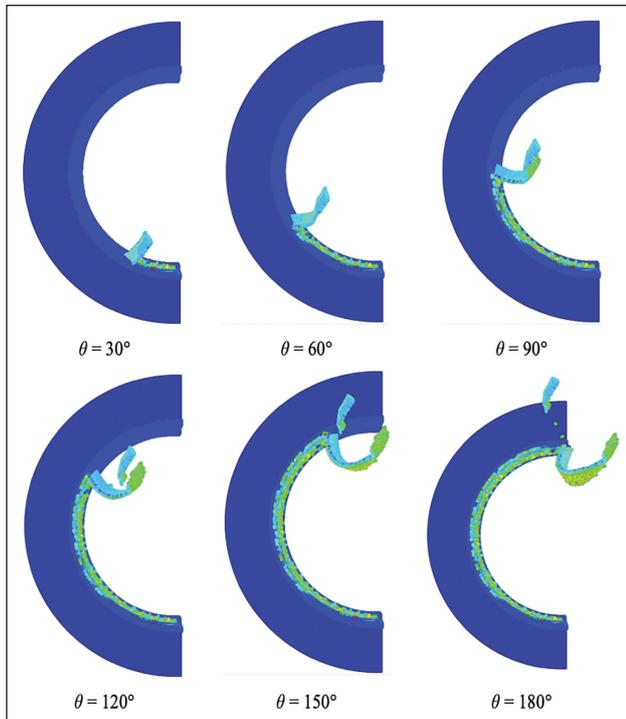
**Figure 4.** Simulation of the chip formation during micro end-milling process according to immersion angle.
