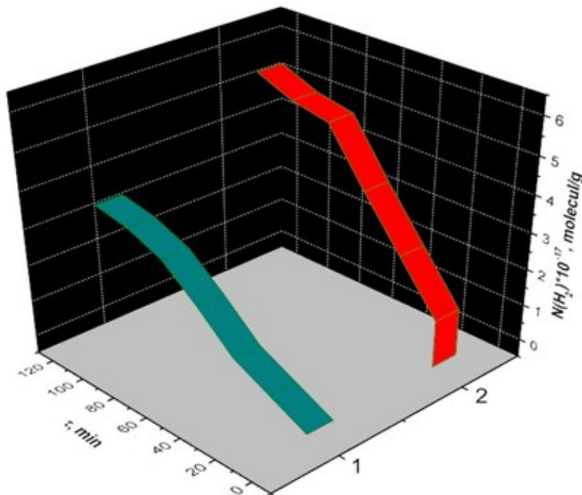
**Figure 1:** Kinetics of the formation of molecular hydrogen during the radiation-heterogeneous decomposition of water in the systems  $(RaO)_x(SiO_2)_y + H_2O$  liquid (1) and adsorbed (2),  $T=300 K$ .
