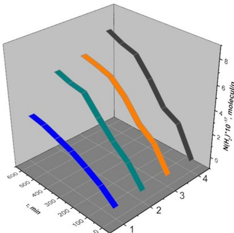
**Figure 3:** Kinetics of molecular hydrogen accumulation during radiation-thermal decomposition of water on the  $(\text{RaO})_x(\text{SiO}_2)_y + \text{H}_2\text{O}_{\text{ads}}$  system at different temperatures: 1-T=373,2-T=473, 3-T=573, 4-T=673 K,  $\rho_{\text{H}_2\text{O}}=5 \text{ mQ/cm}^3$ ,  $D=0,28 \text{ Gy/s}$ .
