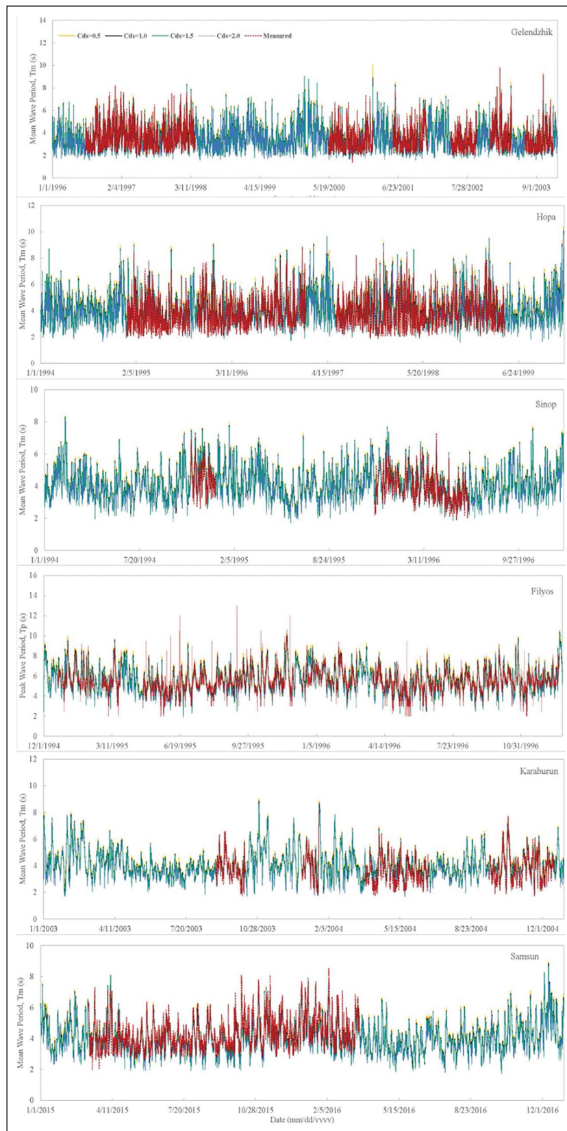
Appendix 6. Comparison between wave period modeled using ERA5 wind fields and measured at Gelendzhik, Hopa, Sinop, Filyos, Karaburun, and Samsun stations.
