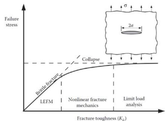
**Figure 1.** Effect of fracture toughness on the governing failure mechanism in a typical brittle material (LEFM: Linear elastic fracture mechanics,  $2a$ : diameter of the crack plate,  $\sigma$ : tensile stress triggering fracture development) [2]
