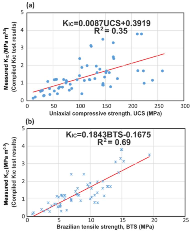
Figure 6. Simple regression models for the evaluation of  $K_{Ic}$  based on different rock properties
