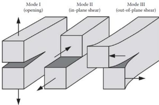
Figure 2. Three fracture toughness models in fracture mechanics [2]
