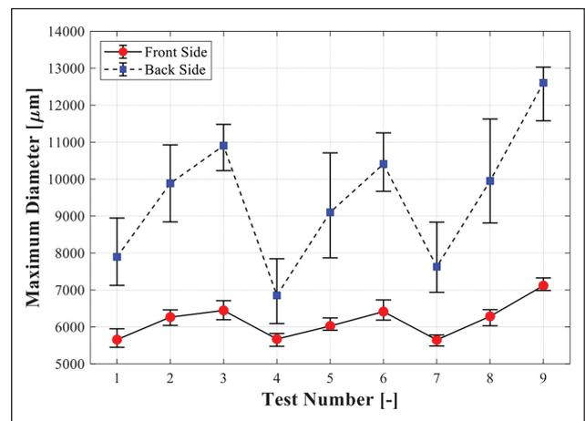
Figure 4. Maximum damaged size on the (a) front and (b) back sides of the composite plate.
