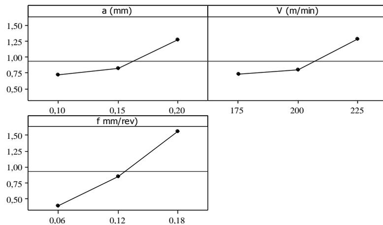
**Figure 5.** The influence of cutting parameters on means response features for surface roughness.
