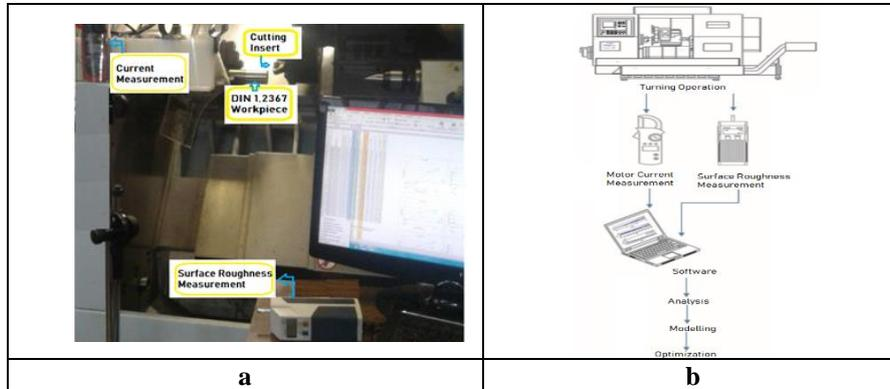
**Figure 4.** a) Experimental setup, b) Schematic diagram in experimental setup.
