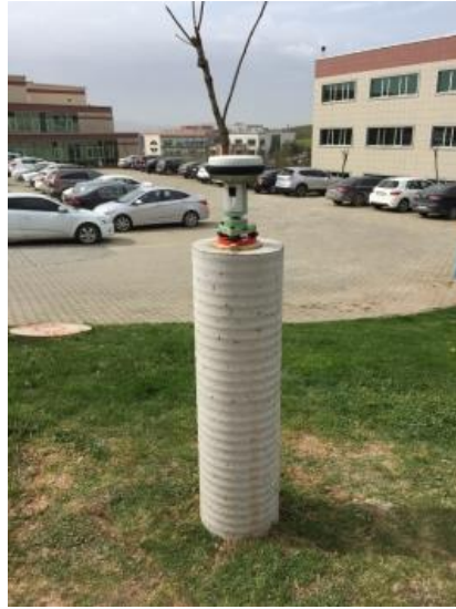
Fig. 3 Established triangulation point (PILYE 1)
