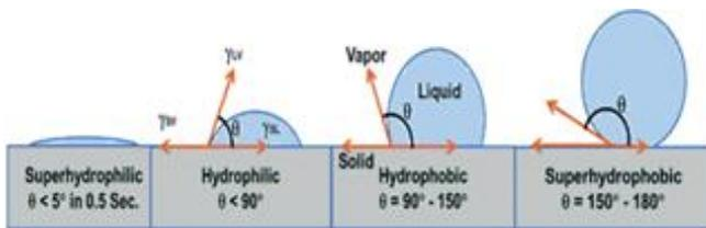
Figure 2. Various conditions according to contact angle of the drop of liquid on the surface [11].
