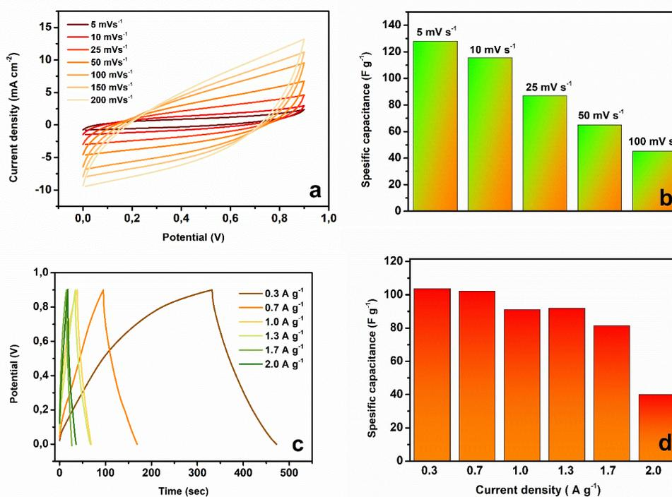
**Figure 4:** a) CVs at different scan rates, b) Specific capacitance values from CVs, c) GCD curves at different current densities, d) Specific capacitance values from GCD of symmetric supercapacitor.
