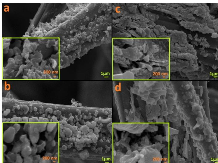
**Figure 2:** The SEM images of a) PANI, b) PANI/AY17, c) PANI/MWCNTs and d) PANI/MWCNT/AY17-3 electrode surfaces.
