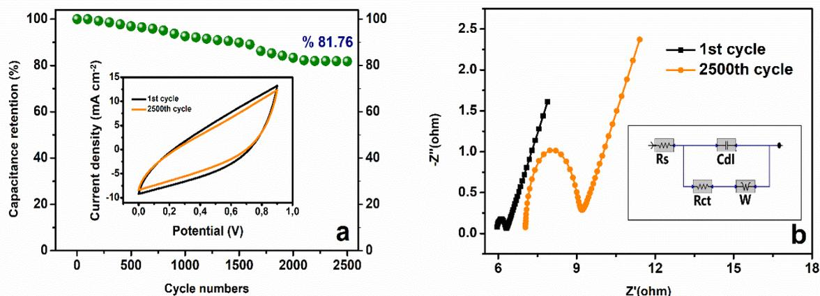
**Figure 5:** a) Long life cycling test of symmetric supercapacitor, b) Nyquist impedance curves of symmetric supercapacitor. The inset is equivalent circuit model.
