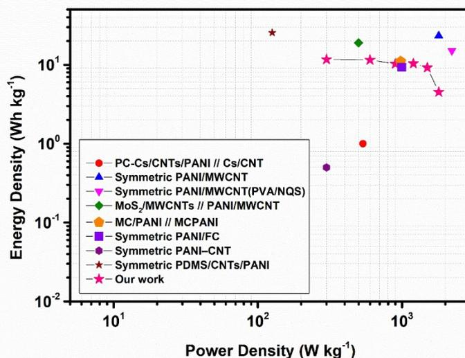
**Figure 6:** Energy density and power density for comparing our supercapacitor in Ragone plot.
