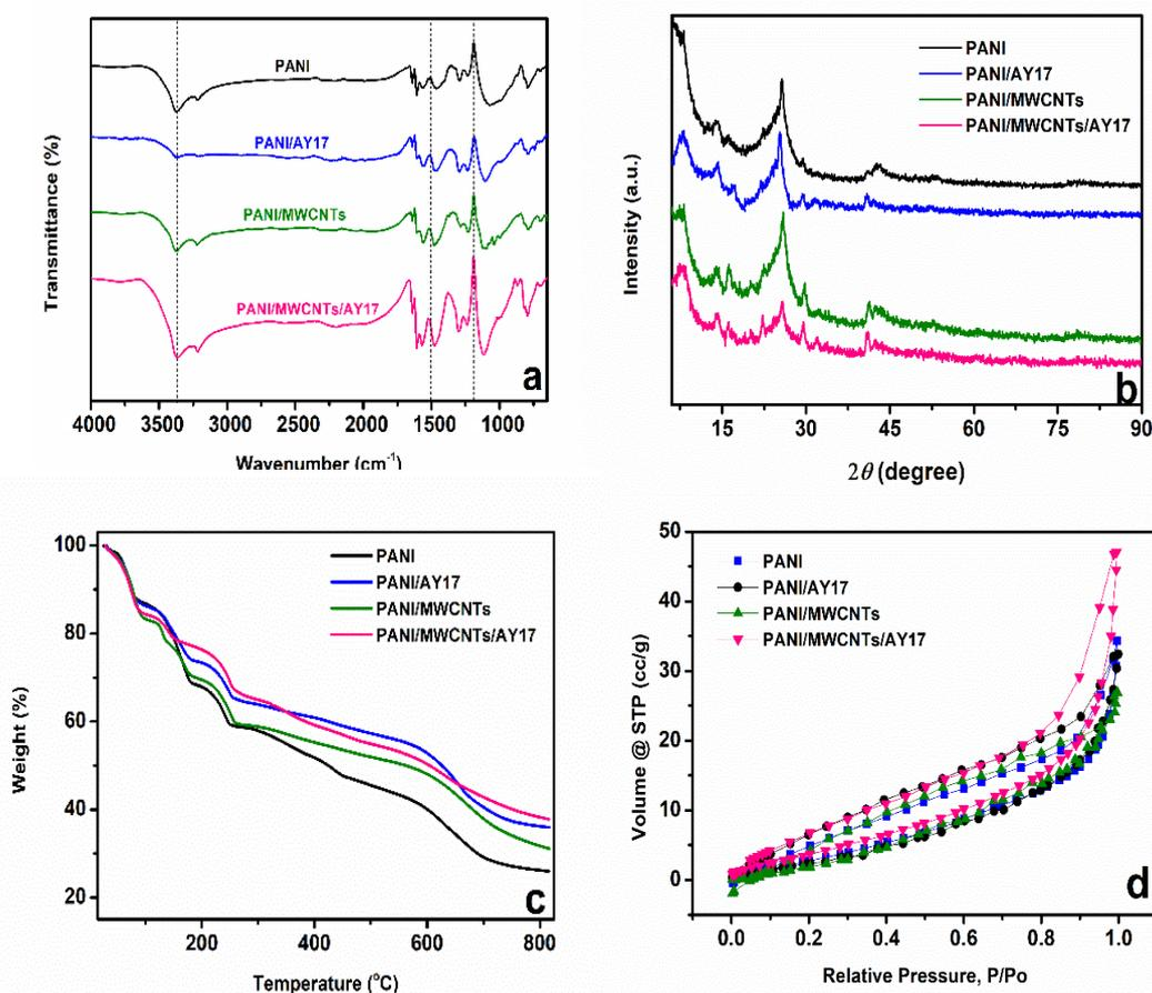
**Figure 1:** a) FTIR analysis, b) XRD patterns, c) TGA curves, and d) N<sub>2</sub> adsorption-desorption isotherms of PANI PANI/AY17, PANI/MWCNTs, PANI/MWCNT/AY17-3 composite electrode material.
