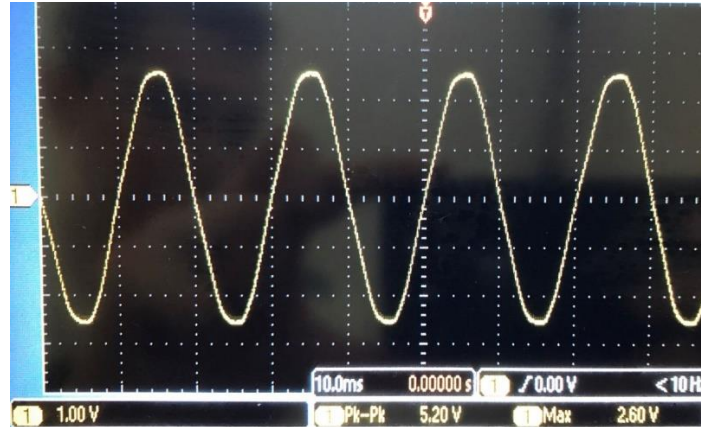
Figure 5. Fault current in the system without R-SFCL
