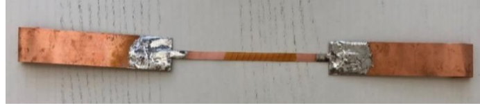
Figure 2. Superconducting tape connection with copper plate
