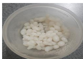
Figure 2. A photograph of a chitosan-based polymer particle
