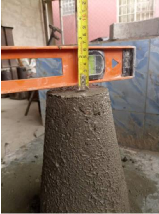
Figure 5. Taking of the slump measurement.
