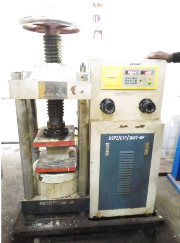
Figure 6. A concrete cube undergoing compression testing.
