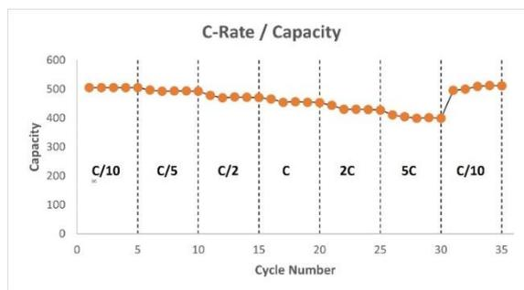
Figure 4 Rate capability of the pouch cell
