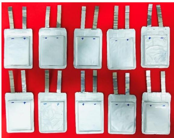
Figure 1 Digital images of pouch cells
