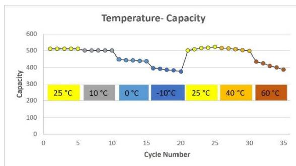
Figure 3 Electrochemical performance of pouch cells at different temperatures
