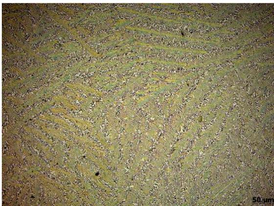
Figure 3. The Optical Micrograph Of As-Cast Alloy.
