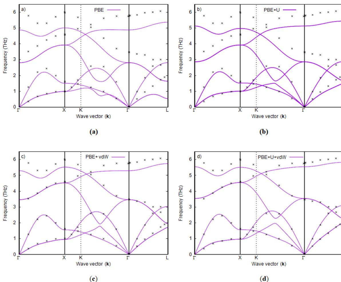
**Figure 1.** Phonon dispersion relations of AgCl along with high symmetry points of the Brillouin zone for a) PBE, b) PBE+U, c) PBE+vdW and d) PBE+U+vdW. Experimental results (cross dots) are taken from neutron neutron scattering measurements of (Vijayaraghavan et al., 1970)
