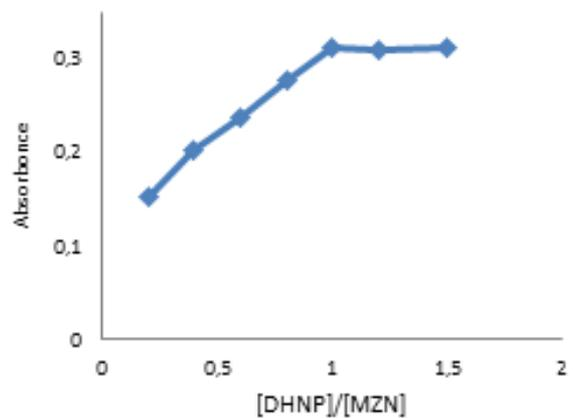
Figure 6. the stoichiometry of the reaction by a) job's method b) mole ratio.
