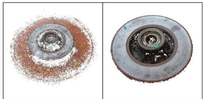
**Figure 11.** Sparse and dense point cloud data (rear)
