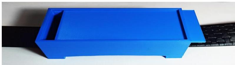
Figure 5. The plastic enclosure case
