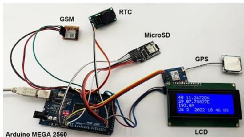
Figure 4. The components of the smart collar
