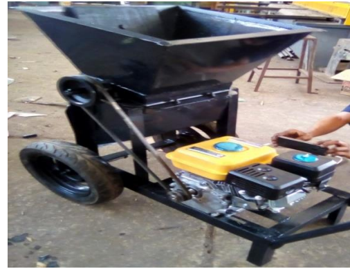
Fig. 4. Developed cassava grating machine
