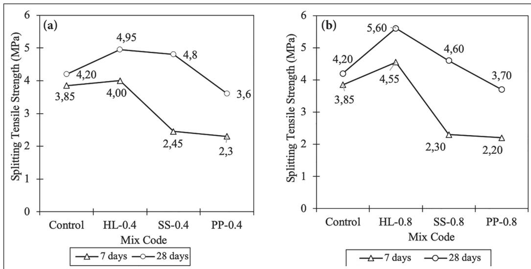
Figure 5. Effect of fiber type and shape on splitting tensile strength for (a) 0.4% volume of fiber, (b) 0.8% volume of fiber.
