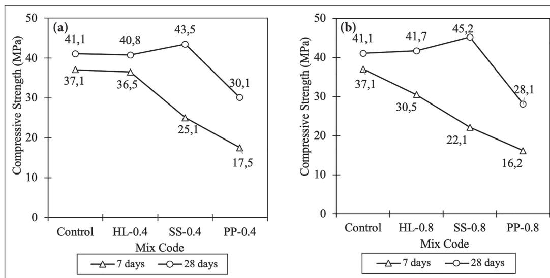
**Figure 3.** Effect of fiber type and shape on compressive strength for (a) 0.4% volume of fiber, (b) 0.8% volume of fiber.
