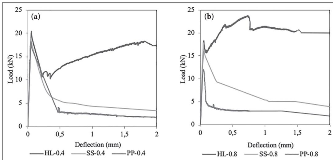
**Figure 10.** Effect of fiber type and shape on load-deflection curves for (a) 0.4% volume of fiber, (b) 0.8% volume of fiber at 28 days.
