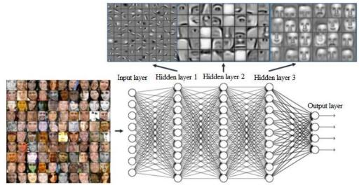
Figure 1. Features obtained for face recognition application in hidden layers of CNN [9].
