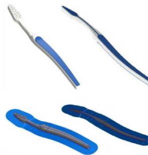
Figure 1 The solid model and parting line of the molded two-component toothbrush
