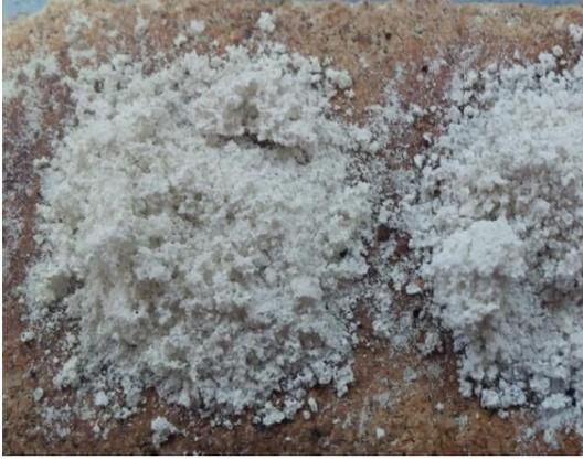
Figure 2. The collapsed HAp foams
