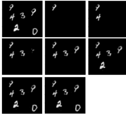
Figure 6. An example MNIST reconstruction result. The top-left image is the original image. The following ones show the canvas after each read/write iteration.
