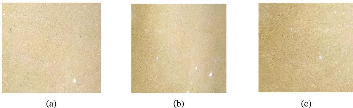
**Figure 2.** Plantain stems; (a) 5% of NaOH, (b) 10% of NaOH, and (c) 15% of NaOH
