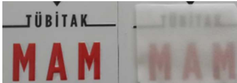
Figure 6. Five layer tapes sintered at 1650 °C.
