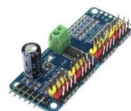
**Figure 6.**PCA9685 16 Channel 12 Bit PWM Motor Driver Circuit [26].
