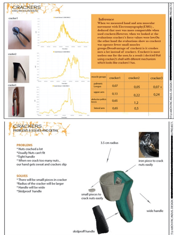
Figure 1. EMG Measurement Results and Functional Evaluation of Three Different Crackers and The Developed Product At The End of The Practice 1
