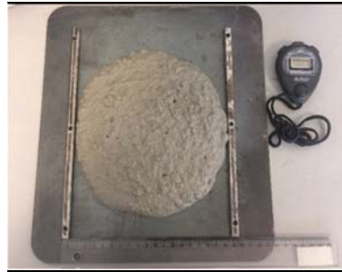
Figure A. Results of self-flow test of the tabular containing MgO based castables
