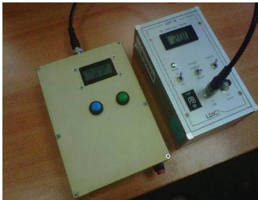
Figure 8. Performance test with LDT-5 PD calibrator tester
