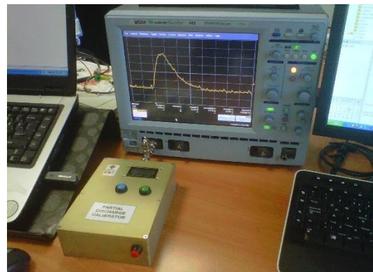
Figure 7. Numerical integration using digital oscilloscope
