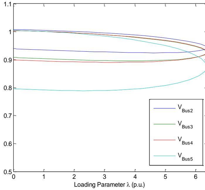
Fig. 6. ( $V - \lambda$ ) Curve obtained bus 2,3,4,5 with connected STATCOM of load bus number 14
