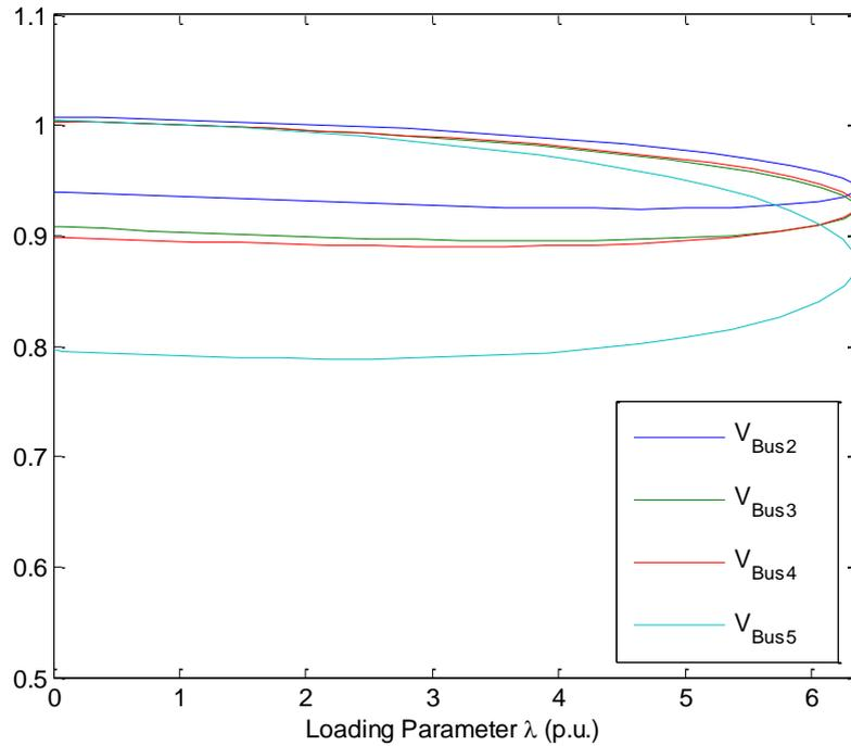
Fig. 10 ( $V - \lambda$ ) Curve obtained bus 2,3,4,5 with connected STATCOM of between buses 6 and 17
