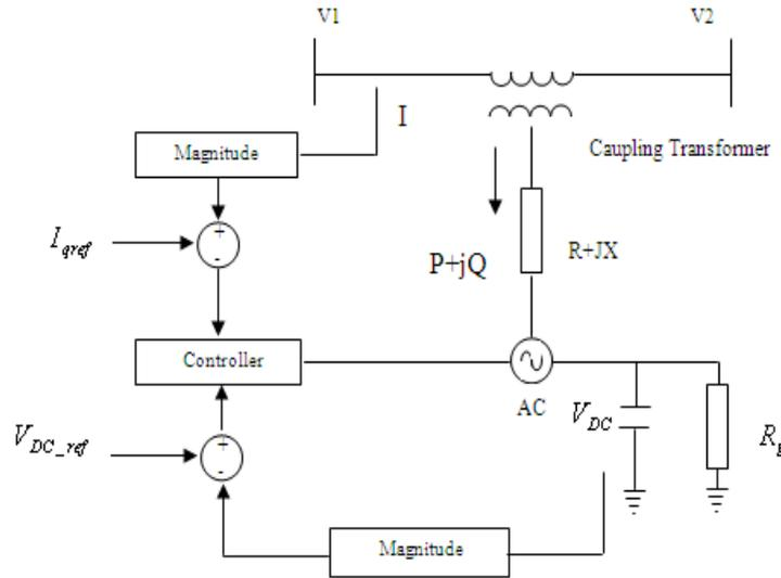
Fig.4. Control model SSSC
