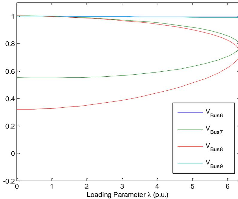
Fig. 11 ( $V - \lambda$ ) Curve obtained bus 6,7,8,9 with connected STATCOM of between buses 6 and 17
