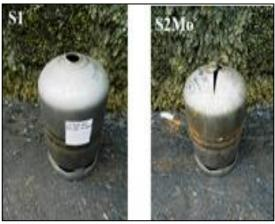
Figure 5. Cylinders subjected to bursting & volumetric expansion test
