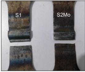
Figure 7. Tensile test specimens. S1 specimen (left), S2Mo specimen (right)
