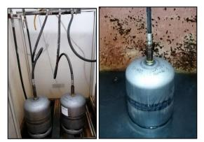
Figure 3. a) Bursting & volumetric expansion test set-up, b) Pressure fatigue test set-up
