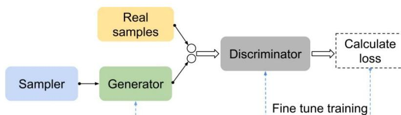
**Figure 1.** The basic schema of GAN architectures.
