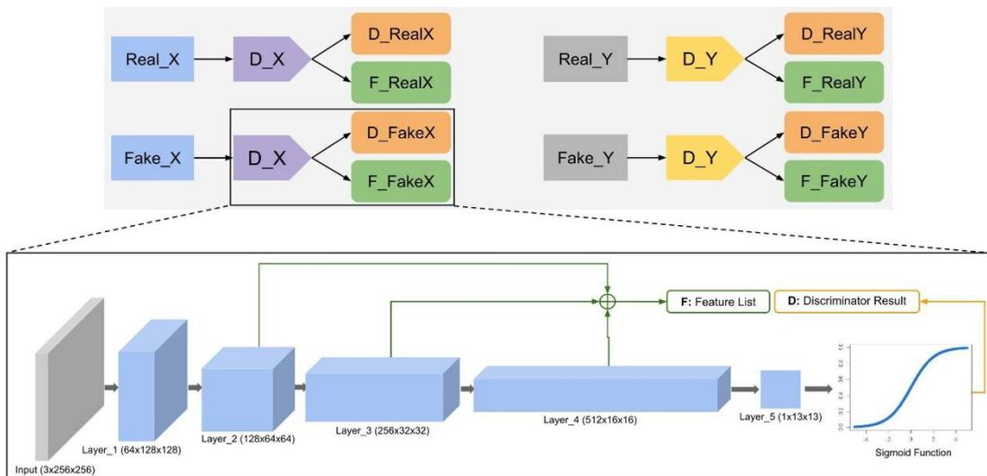
**Figure 3.** The basic schema schematic of DiscoGAN discriminator networks. DiscoGAN’s discriminator  $D_X$  and  $D_Y$  networks learn 2 separate classification processes.
