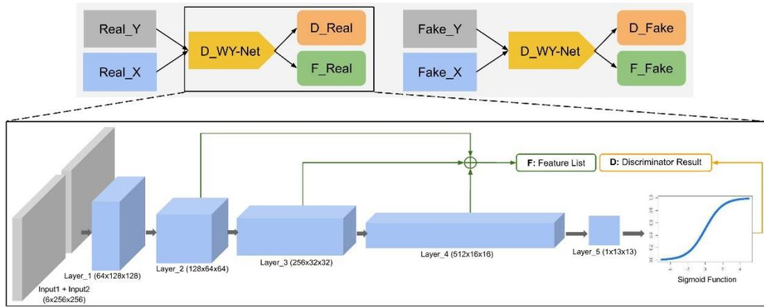
**Figure 5.** The basic schema of WY-Net discriminator network.
