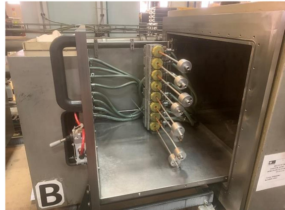
Figure 14. Connecting the samples to the leak tester.
