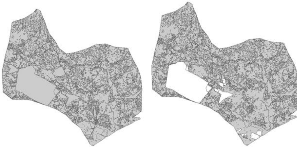
Fig. 4: Integrated method procedure. (a) Merged shapefiles. (b) Dissolved shapefiles
