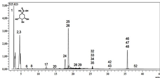
Figure 5. Total ion chromatogram of the lyophilized extract of the plant prepared with water.
