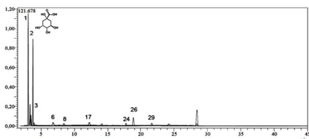
Figure 7. Total ion chromatogram of the lyophilized extract of the leaf of the plant prepared with water.
