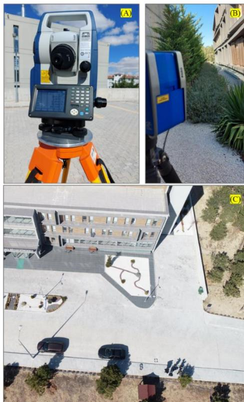
**Figure 3.** Field researches (A: Terrestrial measurements made with the total station, B: Terrestrial measurements made with TLS, C: Measurement with UAS)
