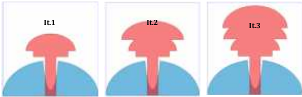
Fig. 2. Three supplementary antenna designing steps
