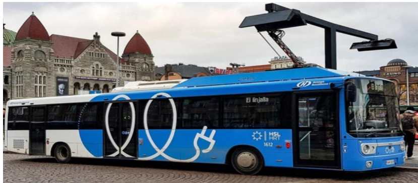
Figure 9. Charging the Electric Bus
