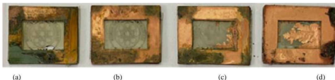
Figure 8. Visual evaluation of nanofibers after: a) 1 min, b) 3 min, c) 5 min, and d) 30 min of electroplating
