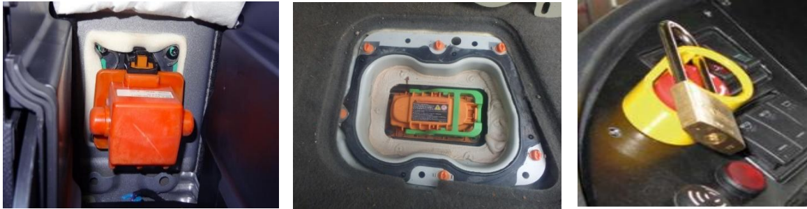
Figure 2. MSD (manuel service disconnect) and emergency stop switches in electric vehicles
