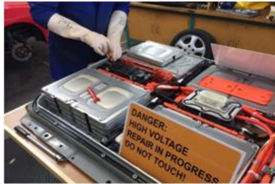
Figure 3. The intervention of high voltage propulsion battery pack used in electric vehicles
