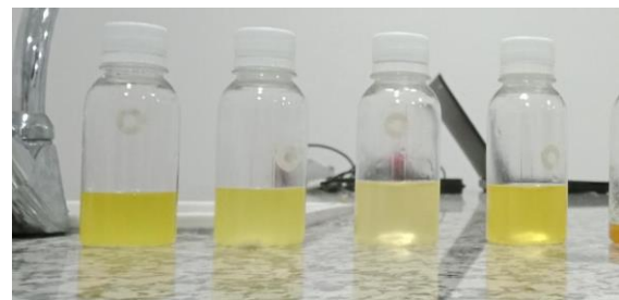
Figure 4. The biodiesels obtained after washing HMP-HSP-HM-HS successively
