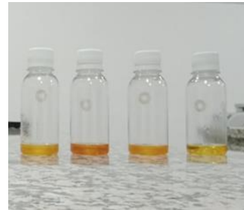
Figure 3. The quantities of glycerine obtained after Separation of (HMP-HSP-HM-HS) successively
