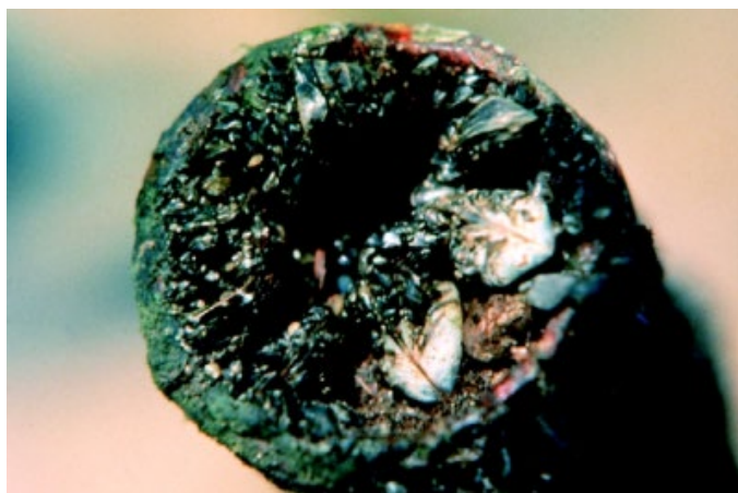
Figure 1. Water intake pipe clogged with adult zebra mussels (de Kozłowski et al., 2002)
