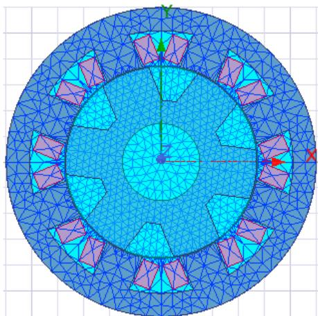
**Figure 2.** Mesh structure of the designed motor
