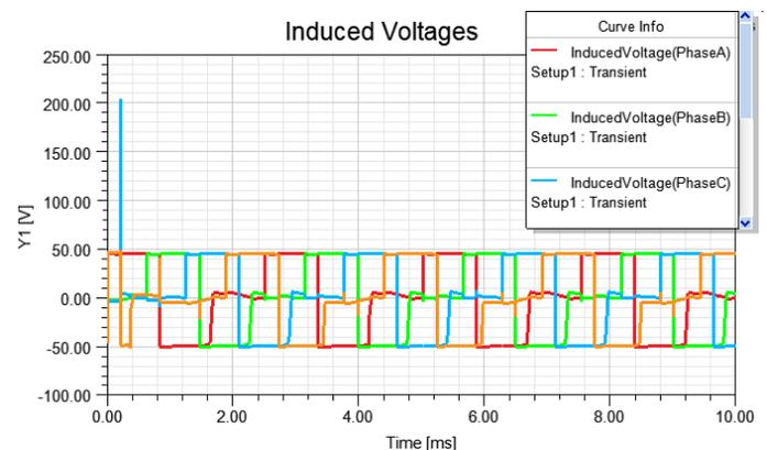
**Figure 8.** Graph of voltage induced in windings
