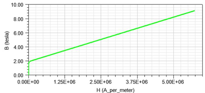
**Figure 4.** Steel 1010 B-H curve used as stator and rotor material
