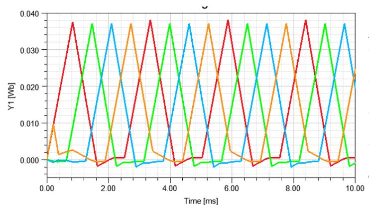
**Figure 9.** Flux values in the windings of the SRM
