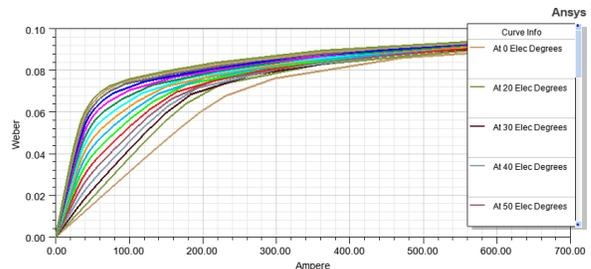
**Figure 7.** Flux-airgap of the SRM
