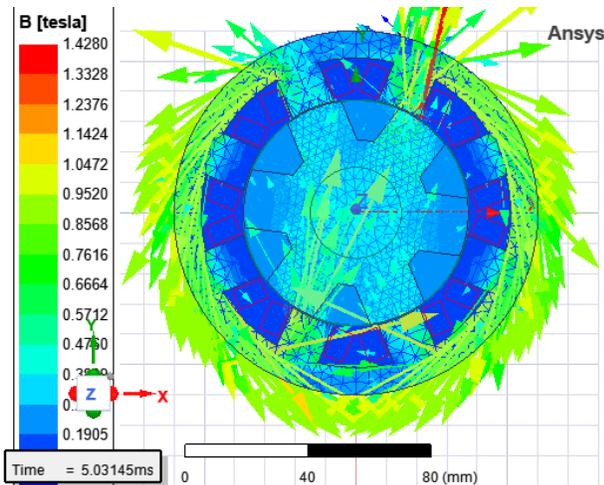
**Figure 5.** Vectorial distribution of magnetic flux values between stator and rotor poles
