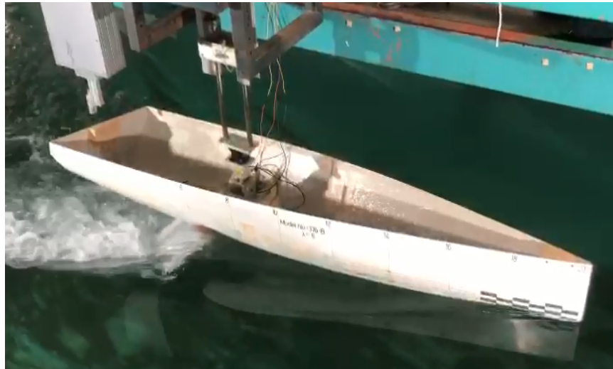
Figure 27: Heeling of the boat with Magnus lift force
