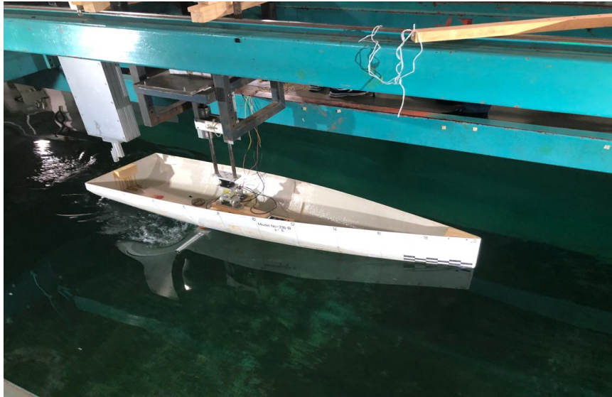
Figure 26: Model boat prepared for towing experiment.
