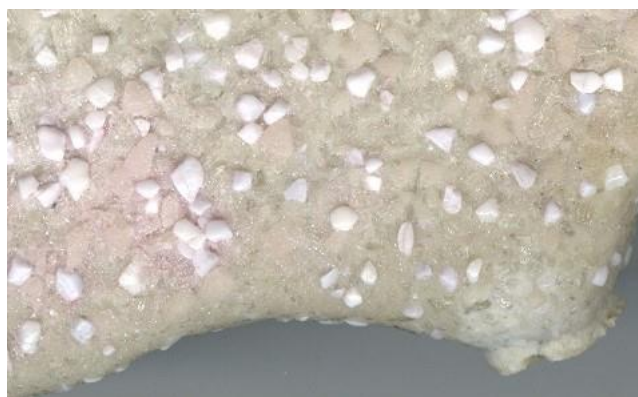
Figure 1. Photograph of corroded refractory brick (GS-M)
