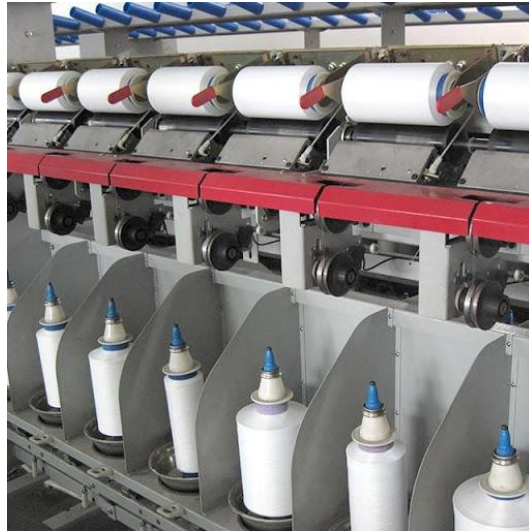
Figure 1. Example of a twister yarn machine [4].
