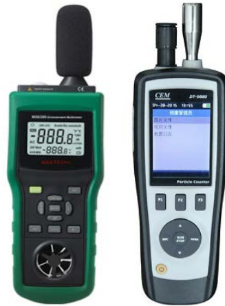
Figure 2. Noise level meter(left) and particle counter device (right)
