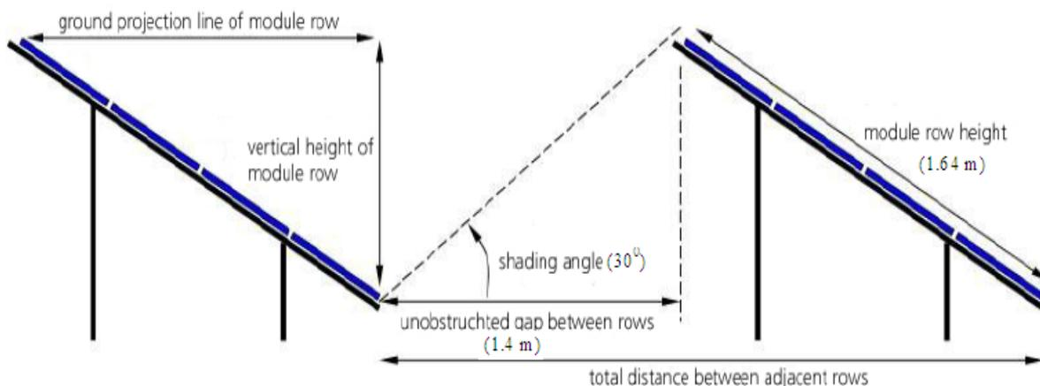
Figure 1. Geometrical Installation of The PV System
