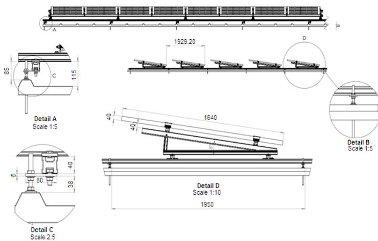
Figure 2. Mounting Diagram of PV Modules
