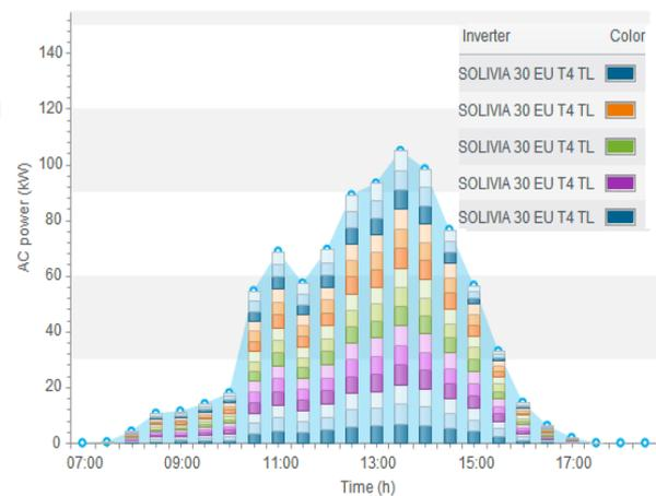
Figure 4. AC Output Power of The Inverter
